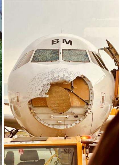
Hail damage on aircraft at Vienna Airport Source: Aviation Security
