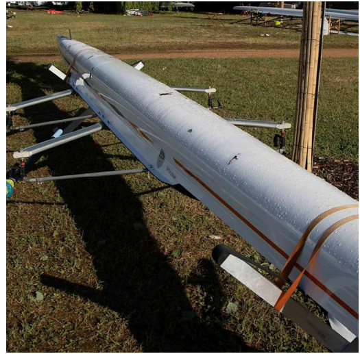
Hail damage on rowboats in Vichy, France Source: Ligue Auvergne-Rhône-Alpes d'Aviron
