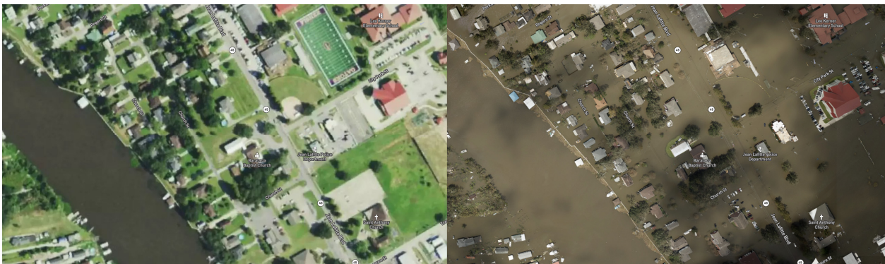
Jean LaFitte: Before (left) and After (right). A levee breach and overtop led to substantial flooding. Source: NOAA
